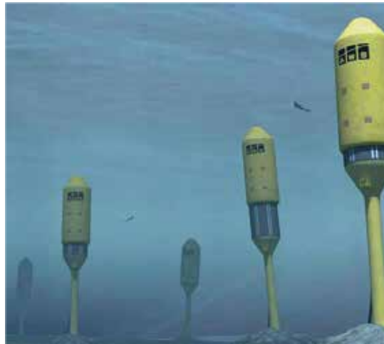
Figure 9 : Submerged Pressure Differential [1]
