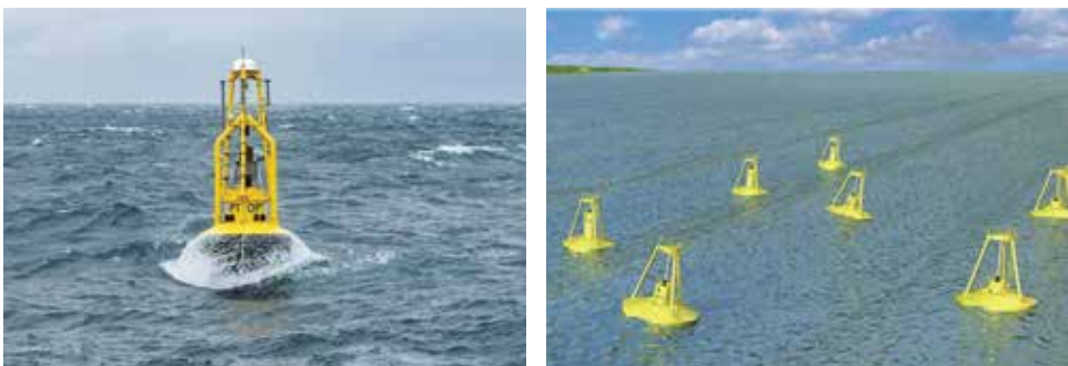
Figure 5 : Point Absorber (Power Buoy) [11]
